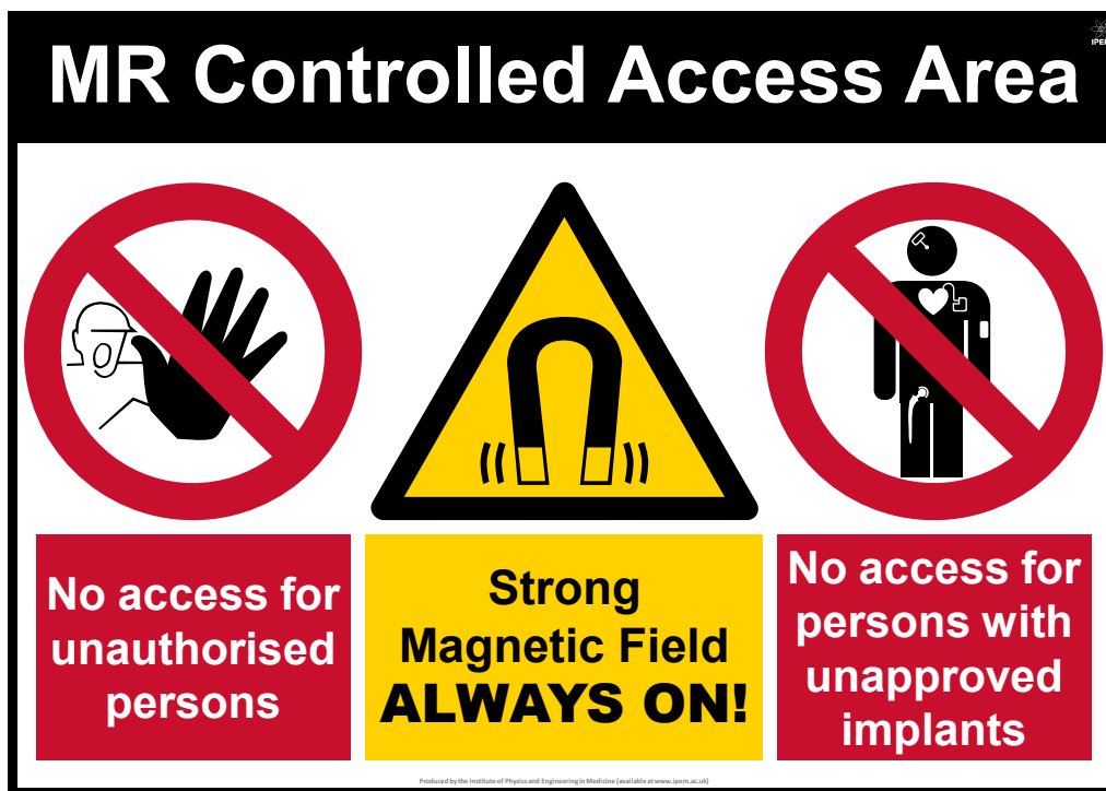
Figure 2: Recommended MRI safety notices for entrance points to the MR Controlled Access Area.
